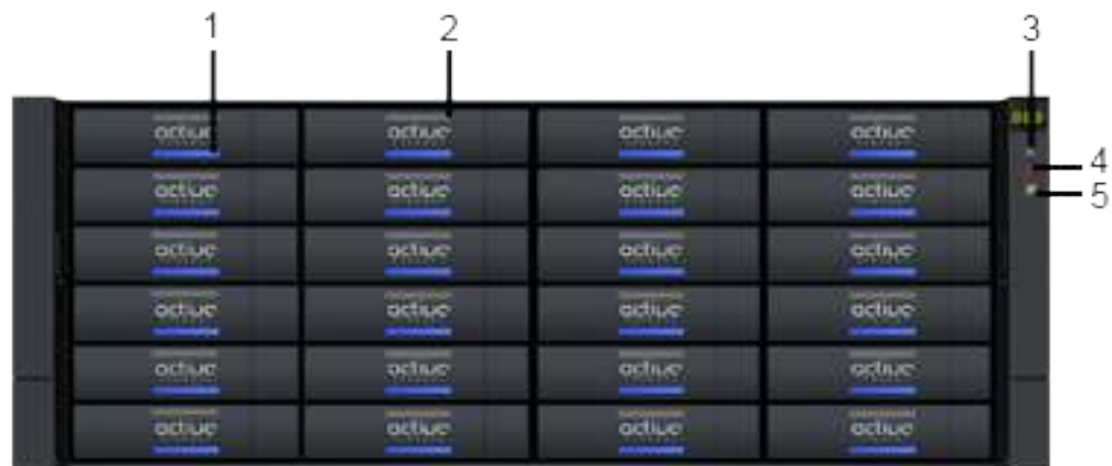
Figure 4-30 Indicators on the front panel of a disk enclosure
