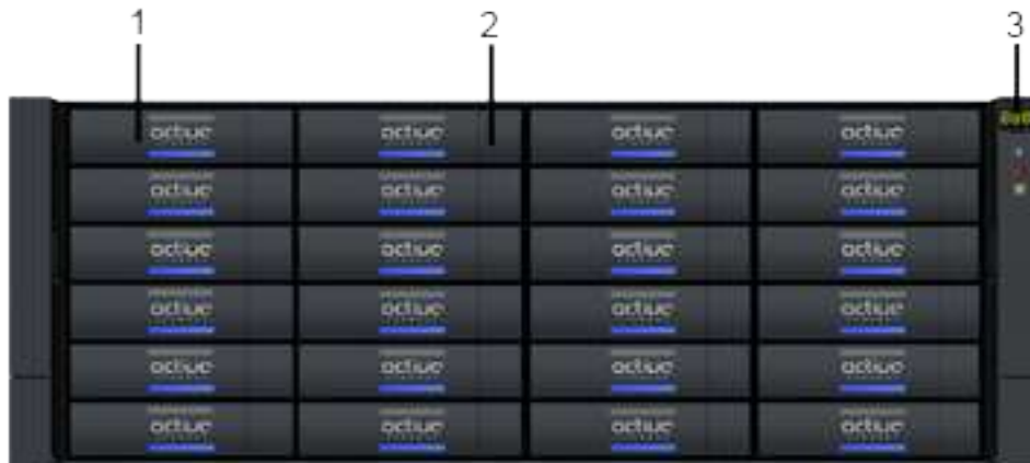
Figure 4-21 Front view of a 4 U SAS disk enclosure
